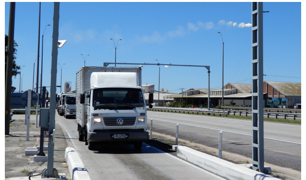
Using LS-WIM for weighing vehicles at a weigh station facility.
